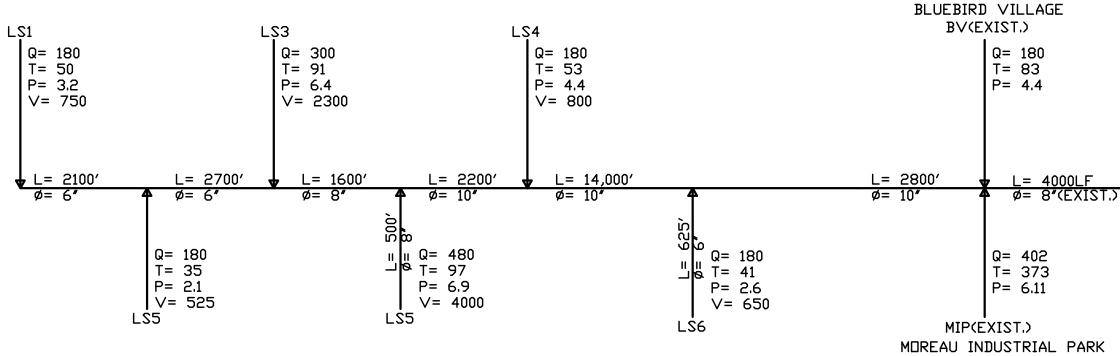
L= SECTION LENGTH OF FORCEMAIN Ø= FORCEMAIN SIZE Q= PUMP RATE (GAL/MIN) T= TOTAL PUMP RUN TIME (MIN/DAY) P= PEAK HOUR PUMP RUN TIME (MIN/20MIN CYCLE) V= AVAILABLE WET WELL VOLUME (GAL) LS1= LIFT STATION & NUMBER
